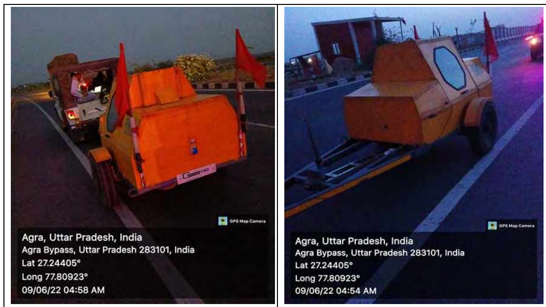
FWD Survey in progress
