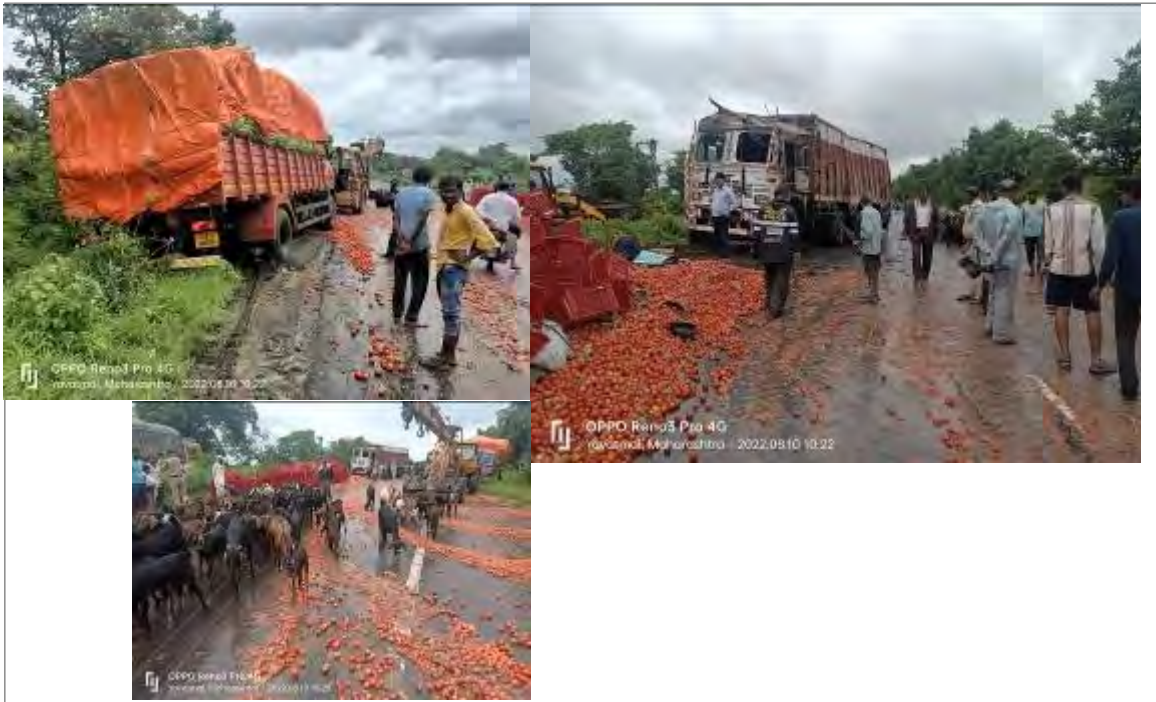
Photo 8: Unbalanced truck accident due to overloading
