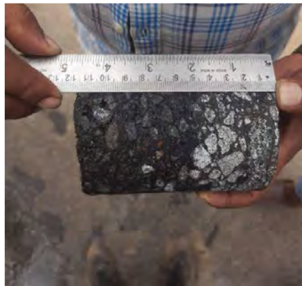
Core Cutting and thickness check at Mananthavady- Kaithakkal Road
