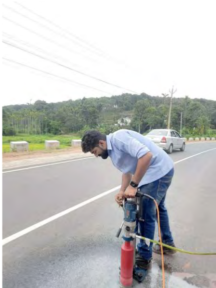
Core Cutting and thickness check at Mananthavady- Kaithakkal Road
