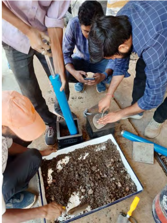
Full Depth Reclamation (FDR) UCS Casting at Pathanapuram-Enath Road
