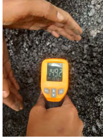
Asphalt Mixing Plant Inspection and Temperature check at Anamala – Chalakkudy Road
